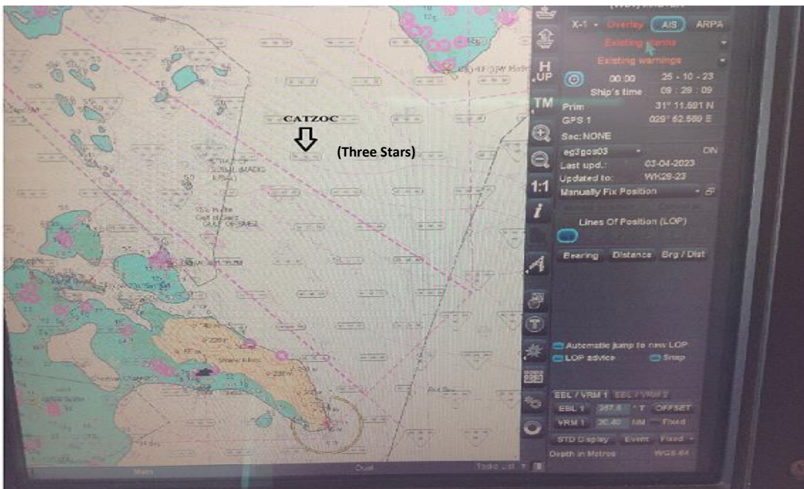
Figure 2: Navigational Danger and Confidence Level of the Electronic Chart in the Gubal Area in the Gulf of Suez Source: Captured from the Transas ECDIS system on the ship "Aida IV"(10/2023)
