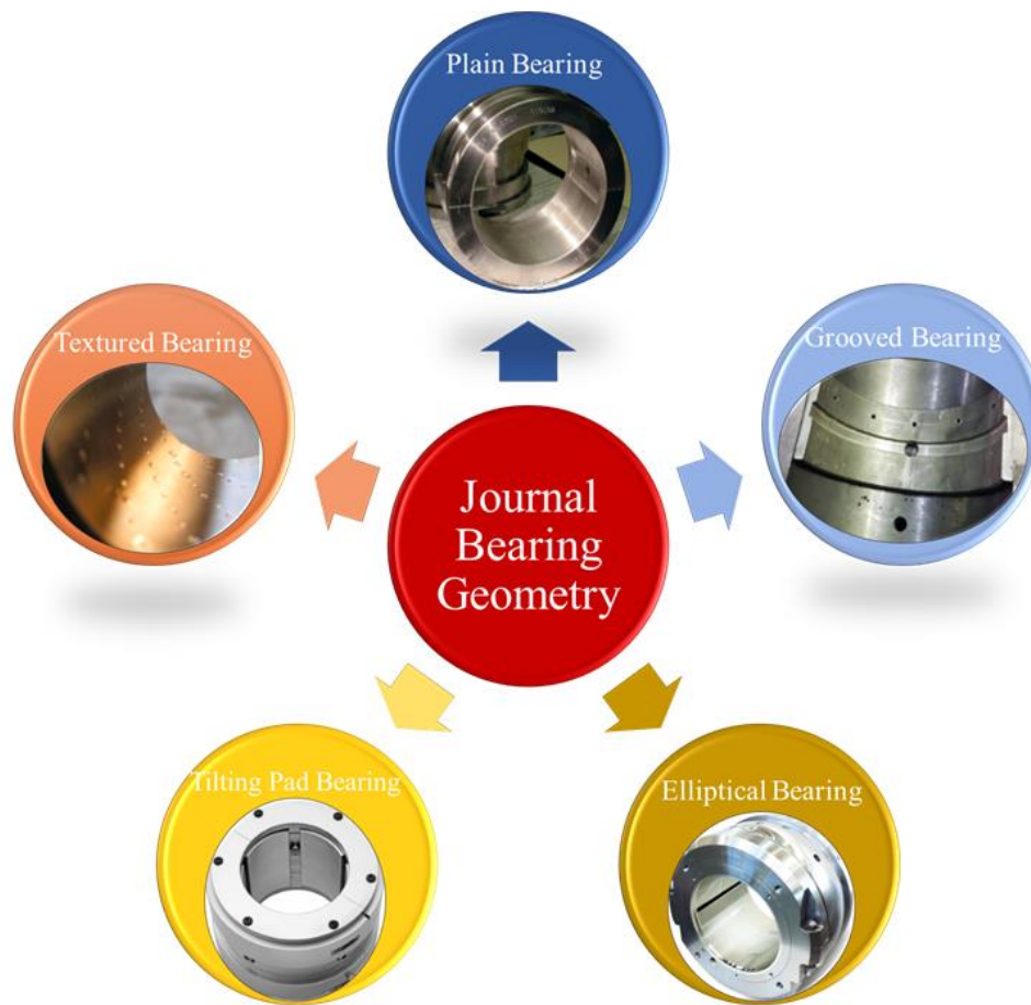
Figure 2: An illustration of different journal bearing geometries. (N. Marey et al., 2021)
